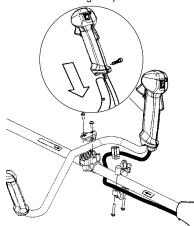
The handlebar mounting must be fitted between the arrows on the shaft.
